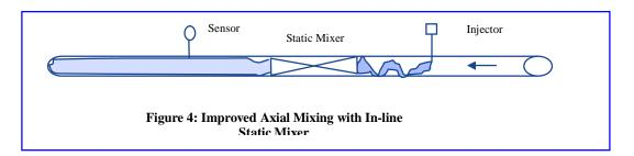
Actual selection of a suitable measurement point may be a process of trial and error. In some systems 10D downstream of the injection point may be sufficient and in others a location as much as 50D may be required. As a general rule, with highly turbulent flow in pipes where there are at least two 90 deg elbows between the injection and measurement points, a separation of 20D is typically sufficient.
