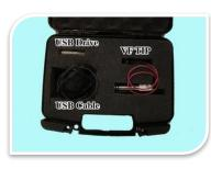
This is metal tip that is used for calibration verification. It has two set calibration standards points with the tolerances and values printed on the tip. It has one switch to transfer between the two set points. One low value and one high value allows you to linearly verify the calibration of the instrument. Comes with a case, USB Drive with software, and a USB Cable.
