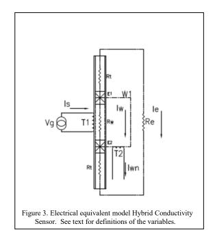
wire tied to the two electrodes to make a direct measurement of the current flowing between the electrodes. That current is determined by the driving potential of the drive transformer divided by the total impedance of the loop, which is overwhelmingly made up of the conductance of the sea water in the cell, the element of interest.
