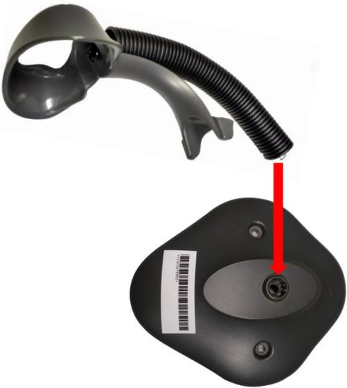
A black barcode reader neck assembly with a flexible black cable is shown above a black base. A red arrow points from the neck's threaded end down to a hole in the base. |
