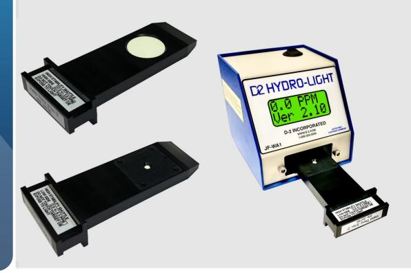
The Hydro-Light comes with the capability to verify the calibration of the device. The calibration remains valid, provided the instrument reads within the printed ranges on each side of the shuttle.
