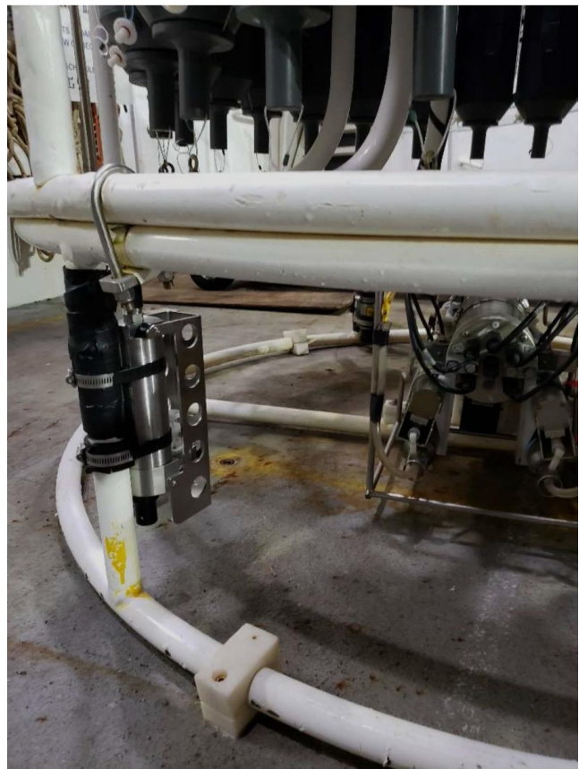
Figure 1: D2 CTD on R/V Endeavor Rosette (4m 5-pin CTD cable used)
