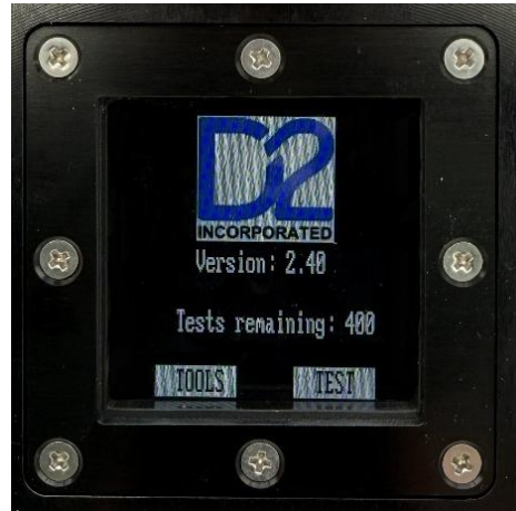
Figure 23. APC Power On Screen
