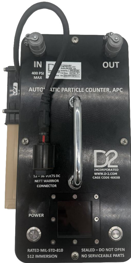
Figure 2. APC (Top View) Powered Off
