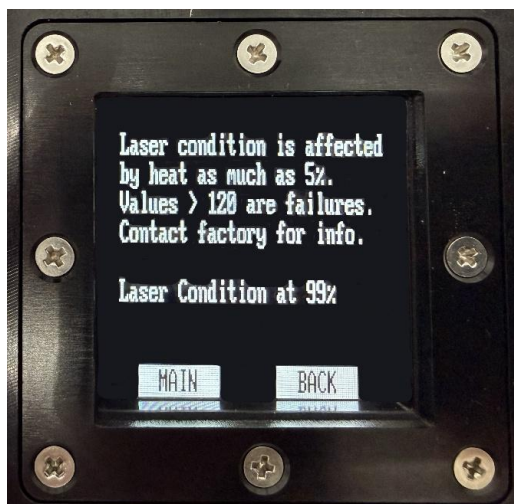
Figure 36. APC Laser Condition Screen
